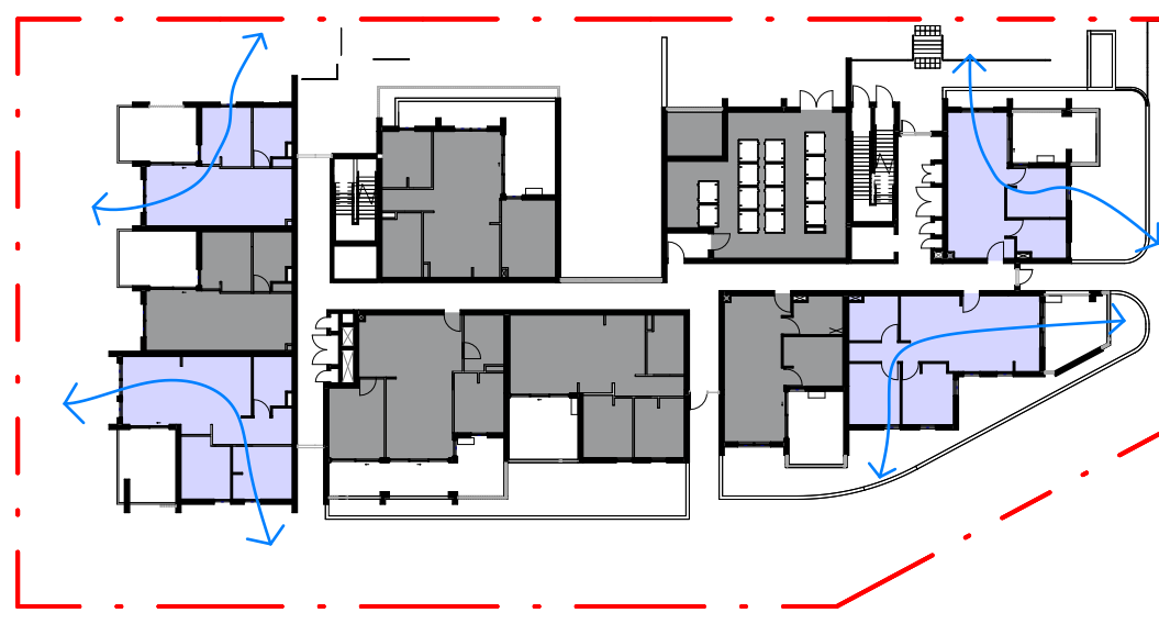
5 CROSS VENTILATION GROUND FLOOR
